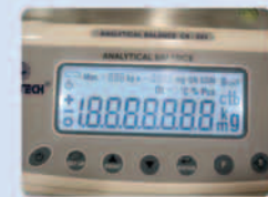
Customized, large, attractive LCD with Multiparameter display illuminated by white backlite
