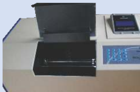
Spacious sample compartment for the convenience of sample handling & cleaning
